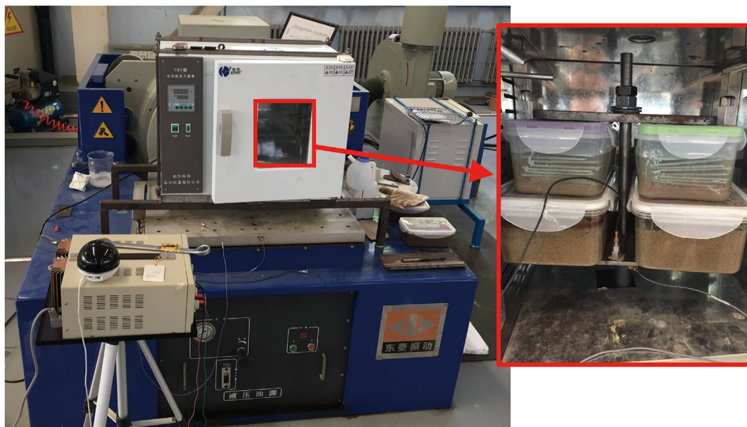
Fig. 5. Coupled temperature and vibration loading experiment process.
